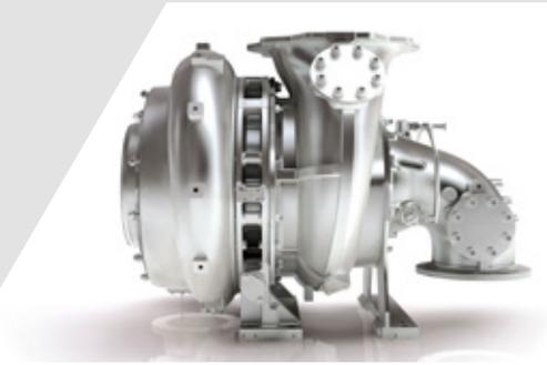
Upgrading the turbocharger of your Wärtsilä 32 diesel engine offers a wide range of benefits and can be achieved in a relatively short timeframe. The Wärtsilä 32 Performance upgrade improves the efficiency, thermal loading, speed margin and turbocharger performance of Wärtsilä W6L32 or W12V32 engines equipped with Napier 297 turbochargers.
