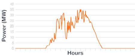
**An illustrative example of a high irradiation day generation from a solar plant**
