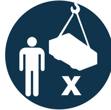
Stay out from under suspended load
