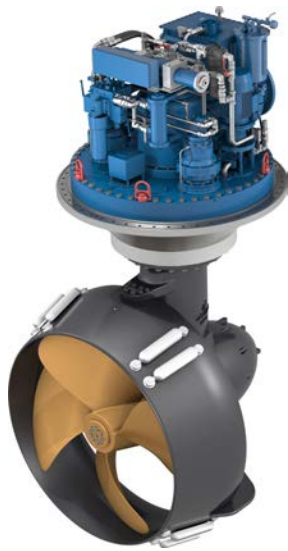
WST with slipping clutch and PTO for diesel-mechanical drive
