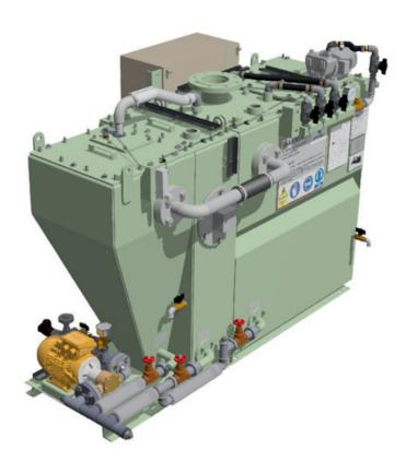
The small ST0-23 sewage treatment plants are our most compact design yet, and they are created to work seamlessly with both gravity and vacuum collection systems, and utilizes the activated sludge system, which speeds up natural biological processes. Chemical chlorination and dichlorination are employed to ensure that the effluent is clean and safe to discharge overboard.
