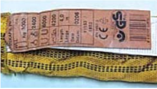
Working load markings are illegible.
