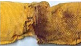
The surface of the webbing sling/round sling has melted due to heat.
