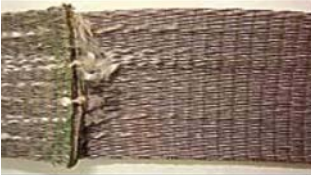
The sling stitching is ripped.
