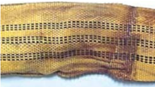
The webbing sling/round sling is worn and dirty or shows chemical damage.
