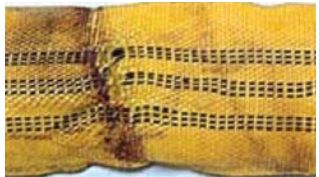
The cut or friction damage exceeds 10% of the sling width.
