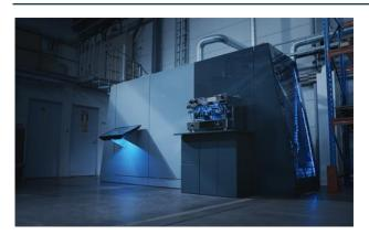
Enabling cleaner air for Wärtsilä employees by returning indoor carbon dioxide levels to those of prehistory. The captured CO<sub>2</sub> can be integrated into an electrolyser and synthesis unit, where it can be converted to fuels or other hydrocarbons.
