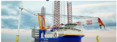
Offshore Wind Installation Vessel being built for Dutch contracting company Van Oord will be powered by five Wärtsilä 32 engines capable of operating with methanol
